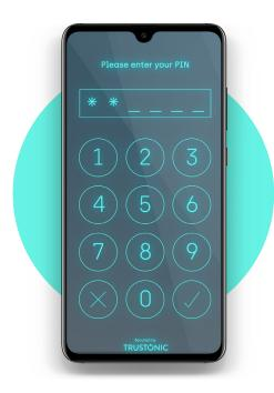
On devices with a hardware-backed TEE and hardware TUI, payment acceptance can be completely isolated from Android. Malware in the Android OS cannot capture the screen, simulate a key press, or spy on what's happening.
